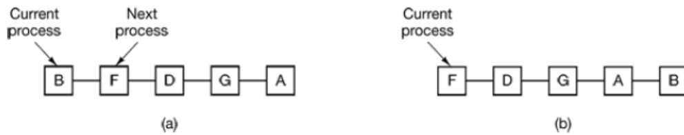
Figure 2-41. Round-robin scheduling. (a) The list of runnable processes. (b) The list of runnable processes after B uses up its quantum.
