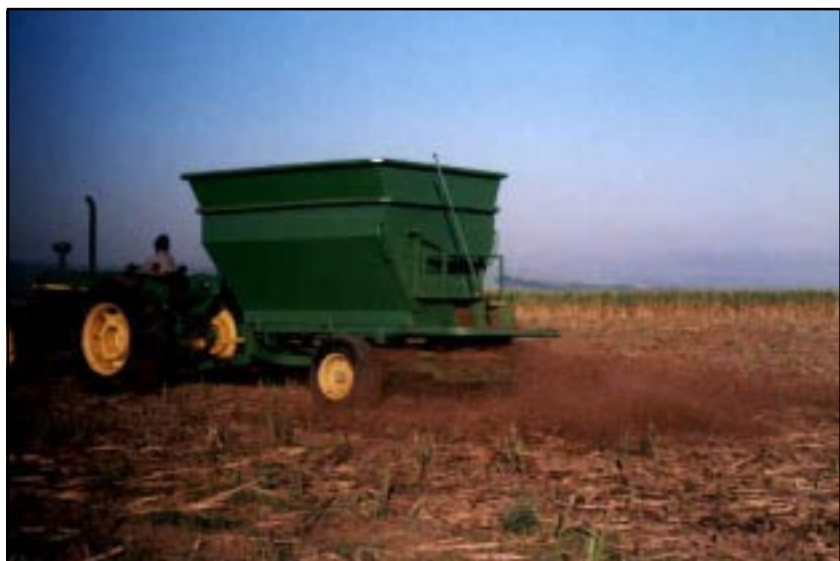
A 'muck spreader' applying chicken litter to sugarcane in the KwaZulu-Natal Midlands.
